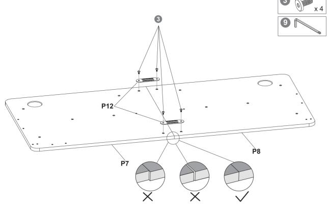
Before tightening the screws, you must ensure that the two desktop pieces are aligned and flush against each other.
